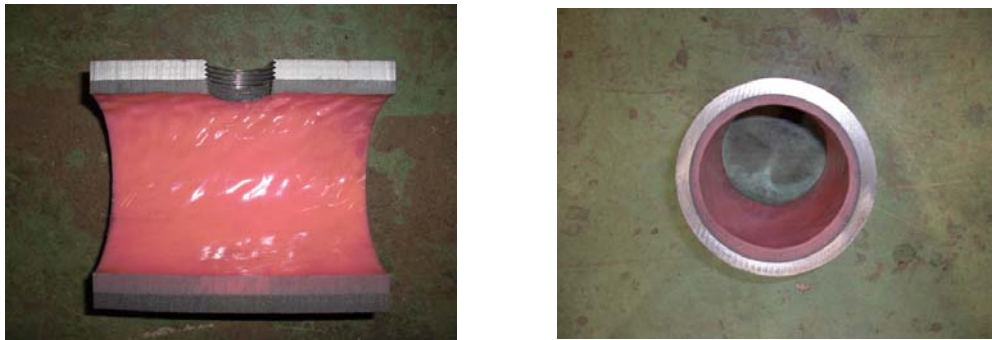
Fig.12 Hole sawing and cutting test
